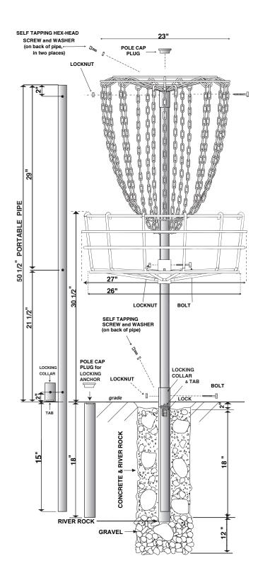
POLE (66 in.) - 1 1/2 in. I.D., 1 15/16 in. O.D. hot-dipped galvanized pipe, drilled.
